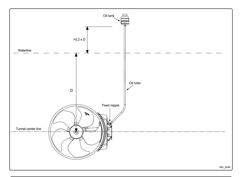
Oil Tank Installation MC\_0023
