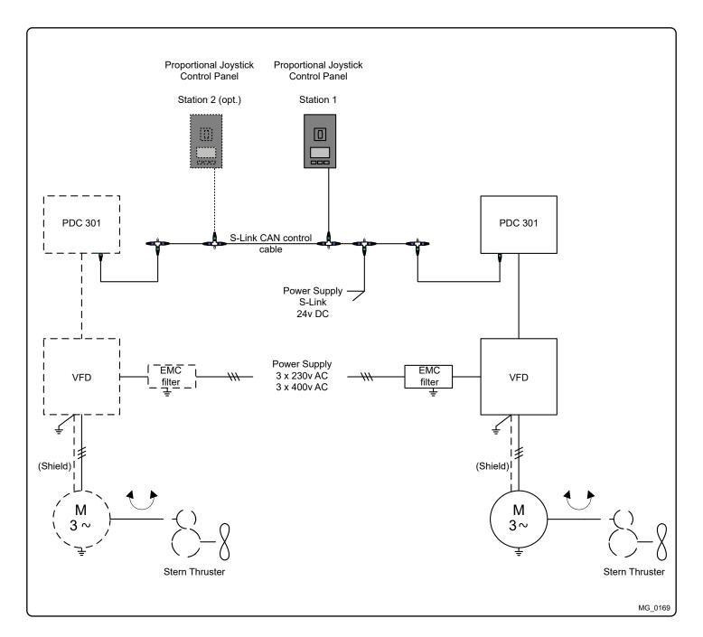
Control Panel Cable Installation
