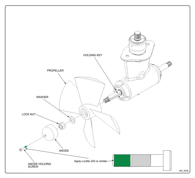
Propeller Installation MC\_0021
