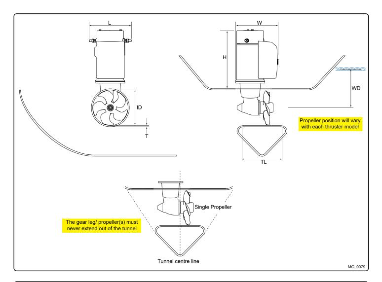
Thruster Measurements MC\_0121
