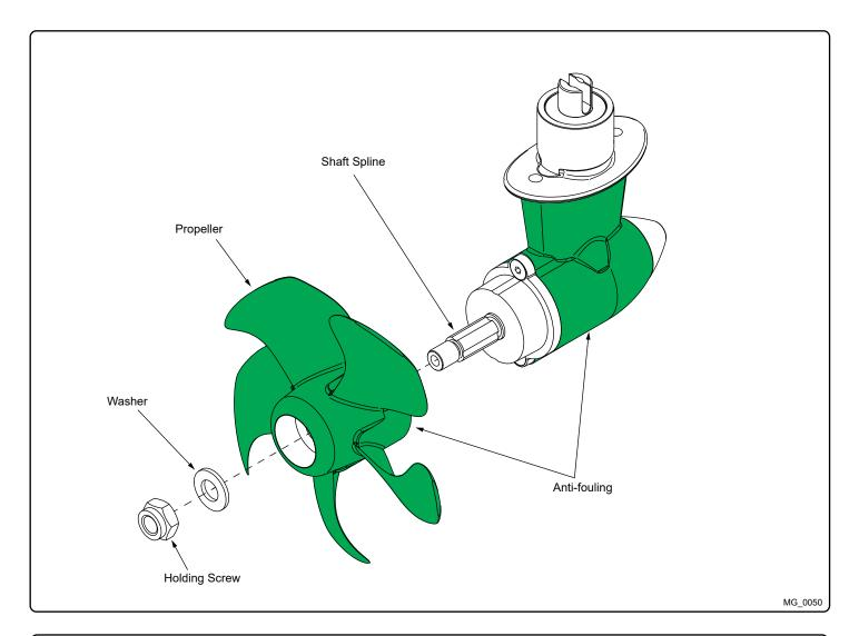
Propeller Installation MC\_0017
