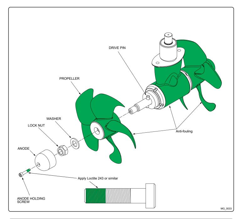
Propeller Installation MC\_0264
