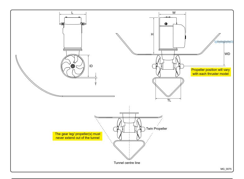
Thruster Measurements MC\_0125
