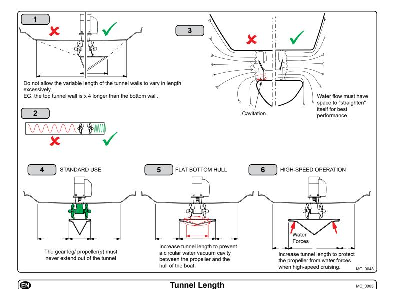
**Optimal tunnel length**Achieving the correct tunnel length depends on many factors from the hull type, operation and environmental conditions.
