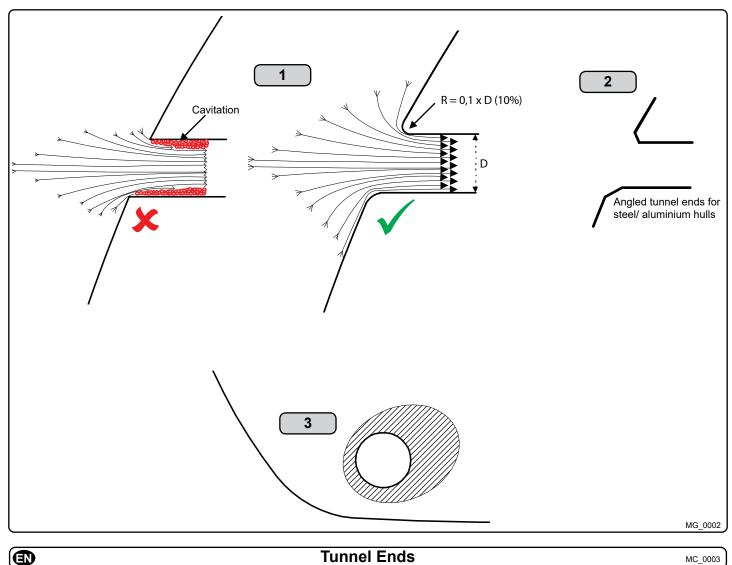
Rounded tunnel ends will maximise thrust and minimise noise and cavitation.
