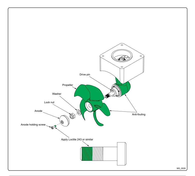
Propeller Installation MC\_0018
