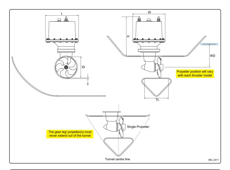
Thruster Measurements MC\_0133
