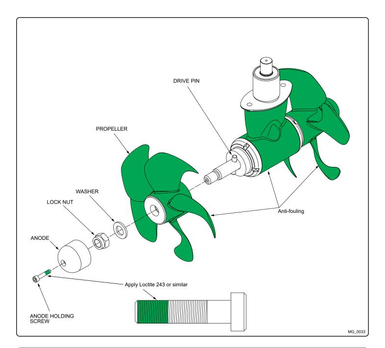
Propeller Installation MC\_0018
