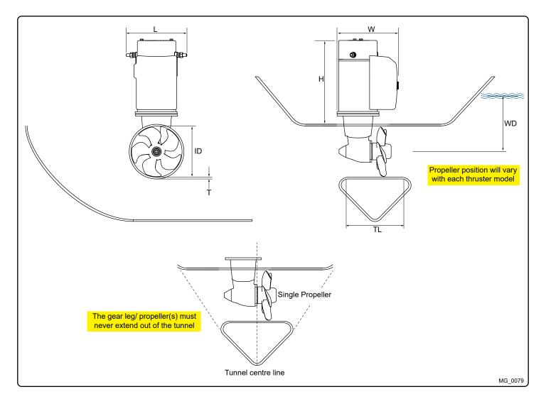
Thruster Measurements MC\_0121
