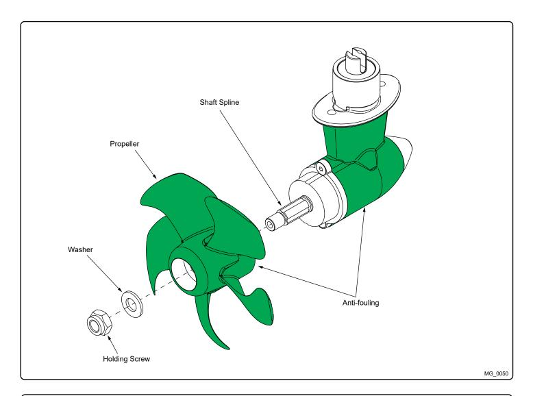
Propeller Installation MC\_0017
