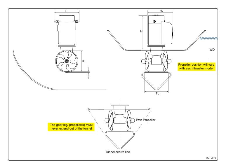
Thruster Measurements MC\_0125
