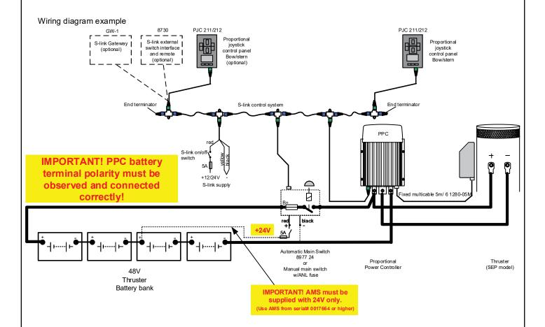
On board charging systems are most commonly 12V or 24V. When charging the 48V thruster battery bank a converter is required. It is the boatbuilder/installer responsibility to arrange this correctly.
