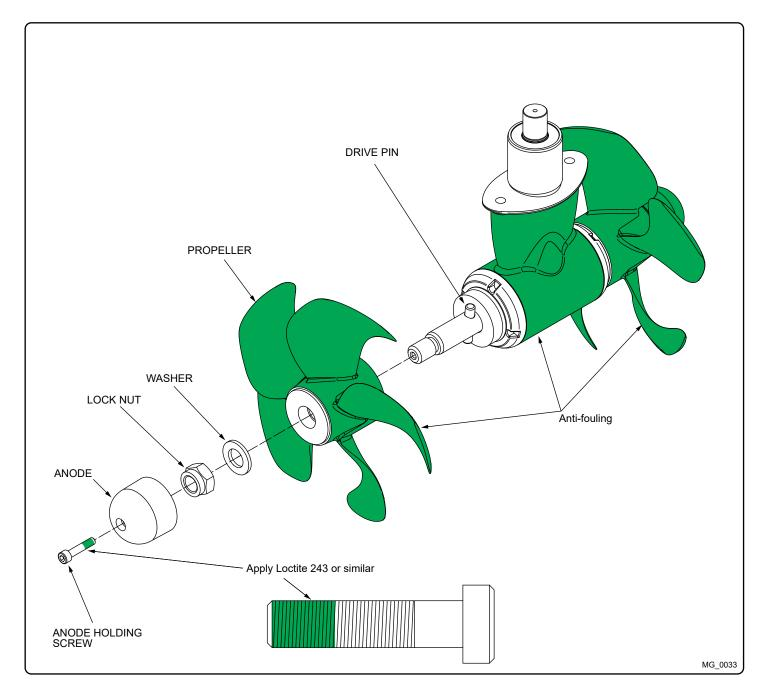
Propeller Installation MC\_0264
