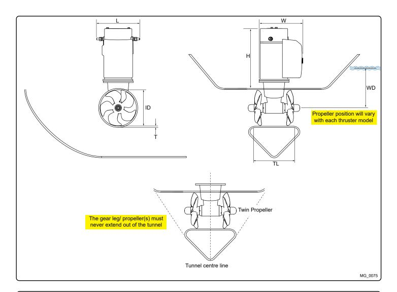
Thruster Measurements MC\_0126
