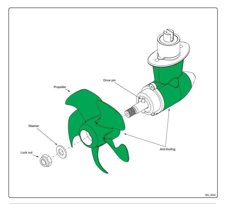
Propeller Installation MC\_0016
