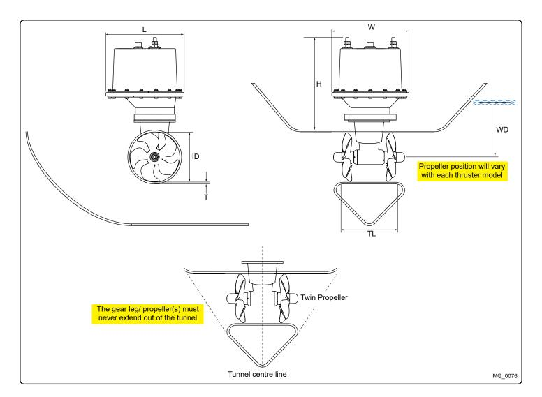
Thruster Measurements MC\_0270
