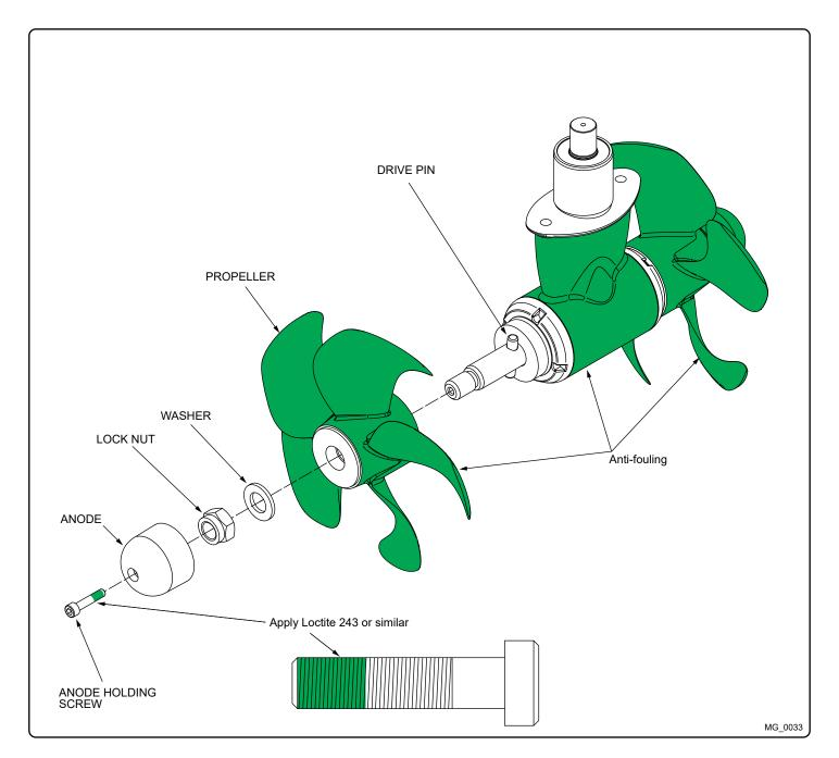
Propeller Installation MC\_0264
