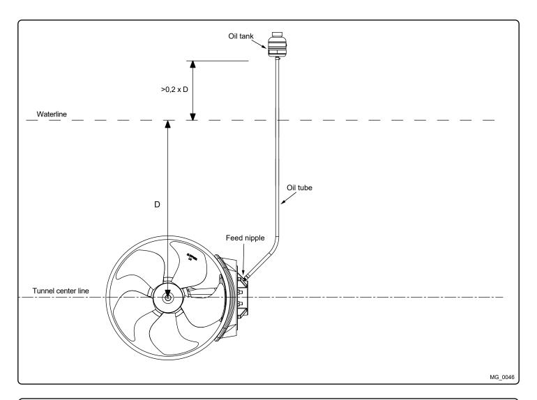
Oil Tank Installation MC\_0023
