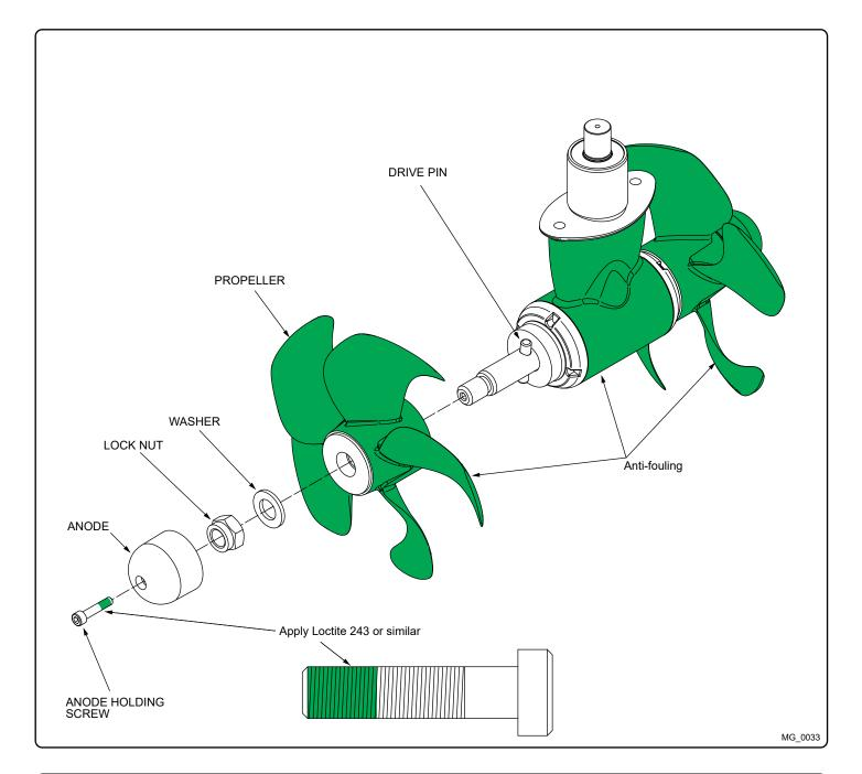
Propeller Installation MC\_0264
