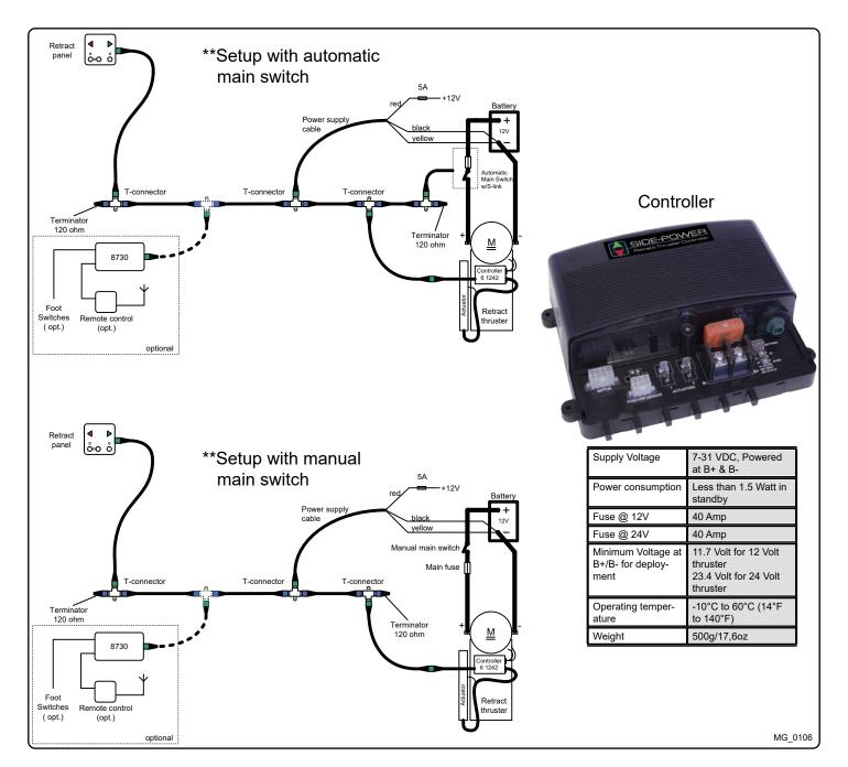
Control Panel Cable Installation MC\_0041
