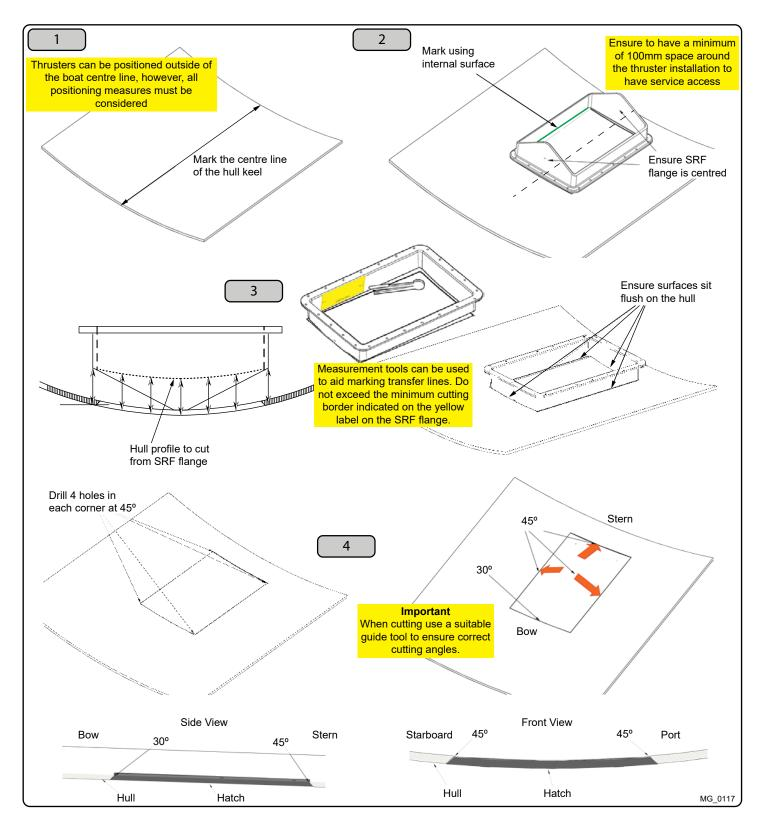
Marking and Trimming of SRF Flange
