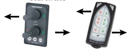
Activating both bow and stern thruster to rotate the boat on axis
